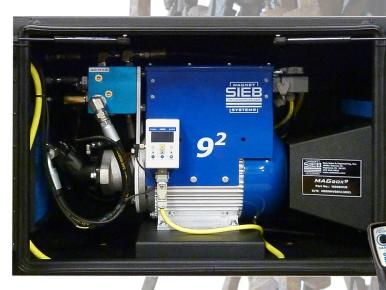
Hydraulic operating parameters: INFLOW 16-18 US GPM @ 2500 psi Max. (Dedicated Pump) 3/4" (I.D.) Min. - High Pressure Hose (P) OUTFLOW 3/4" (I.D.) Min. - High Pressure Hose (T) 3/8" (I.D.) Min. - High Pressure Hose (CD) FLUID TEMPERARUE 125°F Optimum, 140°F Maximum SOLENOID COIL 12/24 VDC (As Required)
