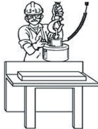
Carefully set the load down. De-energize the magnet by selecting the "PROOF" & "RELEASE." The red indicator light will flash. Hold for two to three seconds; when released the magnet will return to the "OFF" position. Then lift the magnet slightly to be sure the load has been released.
