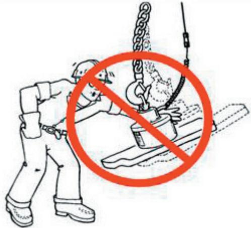
Lift and move the load SMOOTHLY. Avoid jarring and swinging the load while it is in transit. KEEP THE LOAD LEVEL. NEVER let the load come in contact with any obstruction.
